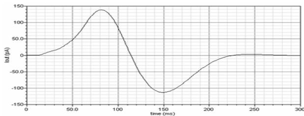
Fig. 6 Wavelet Filter (gauss1) Impulse Response
