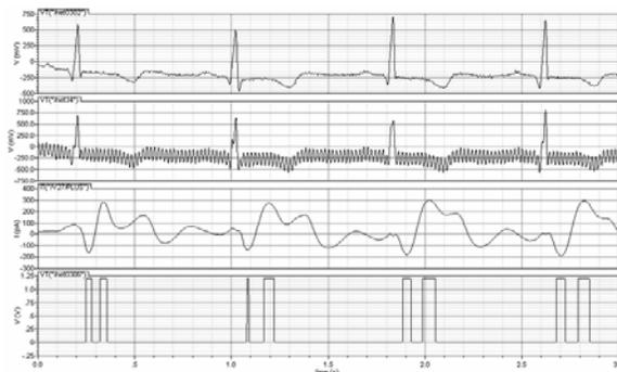
Fig. 9 Transient responses of the wavelet filter (3rd line) and the comparator for a stylistic cardiac signal (1st line) contaminated with 50Hz interference (2nd line)
