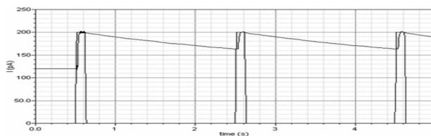
Fig. 8 Transient response of the peak detector
