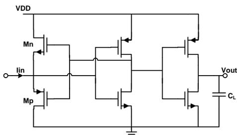
Fig. 5 Comparator Circuit
